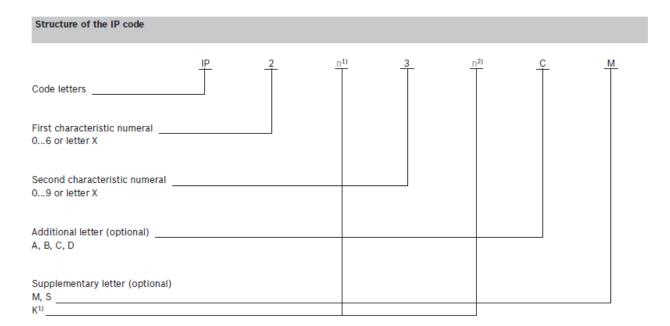
If a characteristic numeral is not given, it must be superseded by the letter "X" (i. e. "XX" if both characteristic numerals are not given). The supplementary and/or additional letters can be omitted at will, and need not be superseded by other letters.
